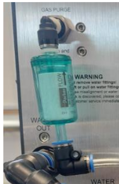
Figure 11: Purge gas connection to an i401 laser.
