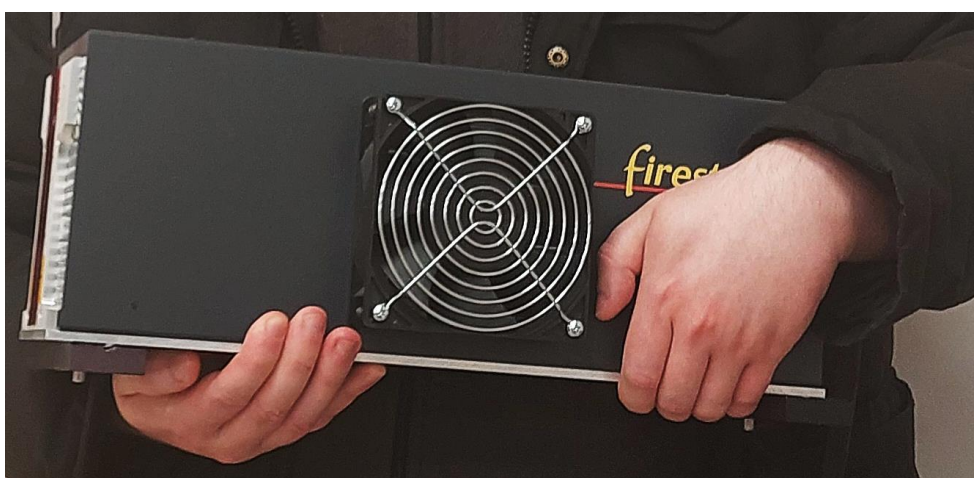
Figure 3: Example of lifting a ti series laser by holding it in the middle, do not carry laser by the mounting feet.
