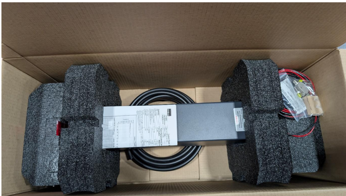
Figure 1: Content of the laser box with laser in the middle, small hardware accessories in the upper right and water tubing at the bottom of the box.
