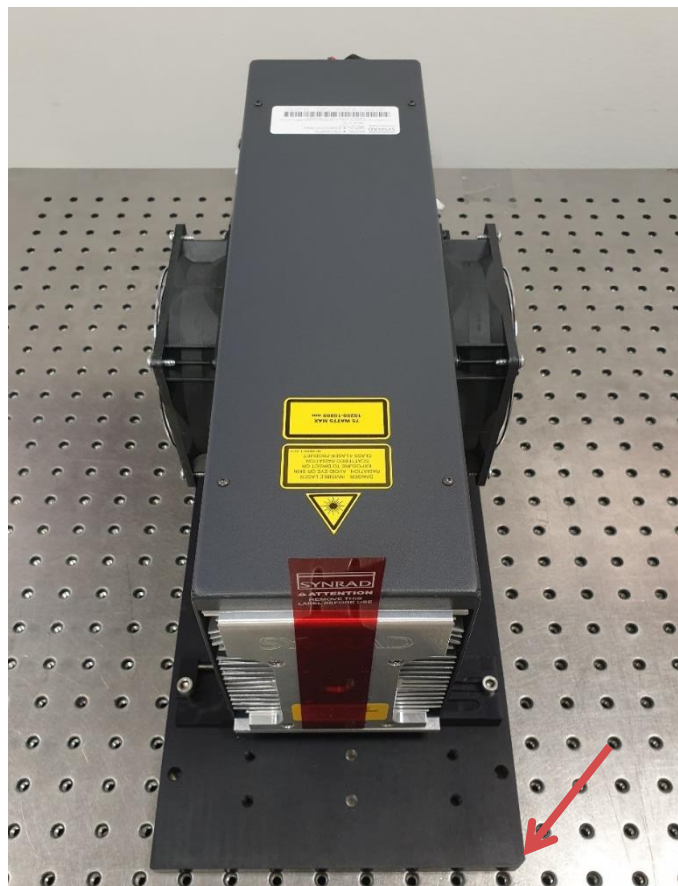
Figure 8: v30 laser fixed on the mounting rail with four 1/4-20 UNC cap screws (the position of the notch is highlighted).
