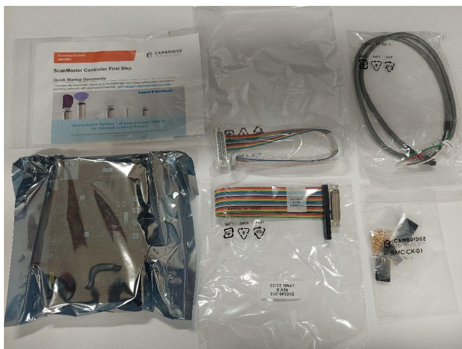
Figure 5: Content of the SMC controller box (clockwise from the upper left)– Flyer with First Steps and Download information, Command Cable, SMC power cable, Hardware accessories (connector kit), Laser adapter cable, ScanMaster Controller.
