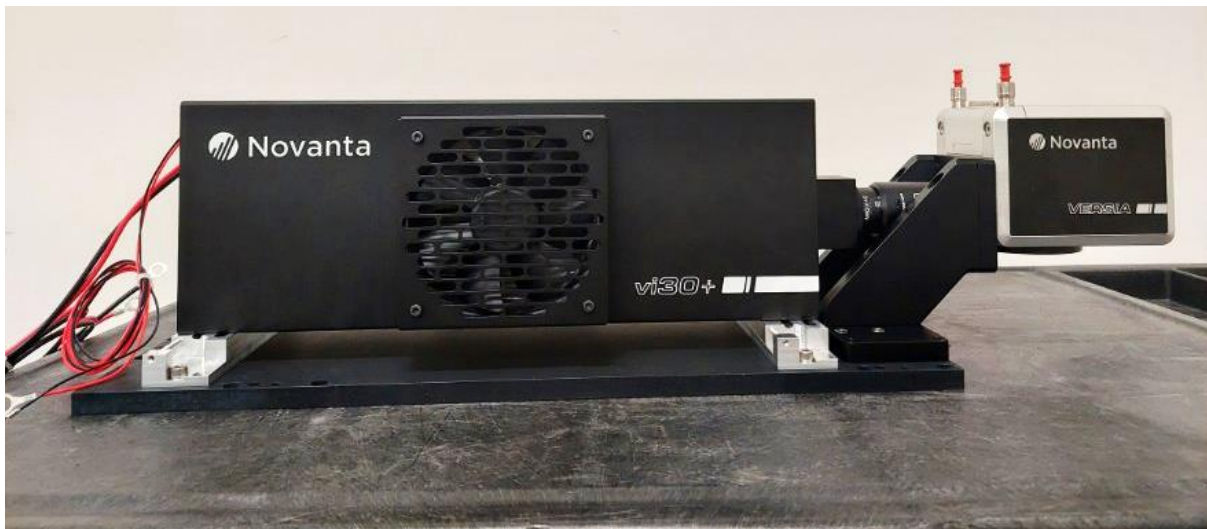
Figure 14: Mechanical mounting of a VERSIA - vi30+ Integrator Package
