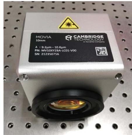
Figure 11: MOVIA scan head with installed lens spacer containing f-theta
