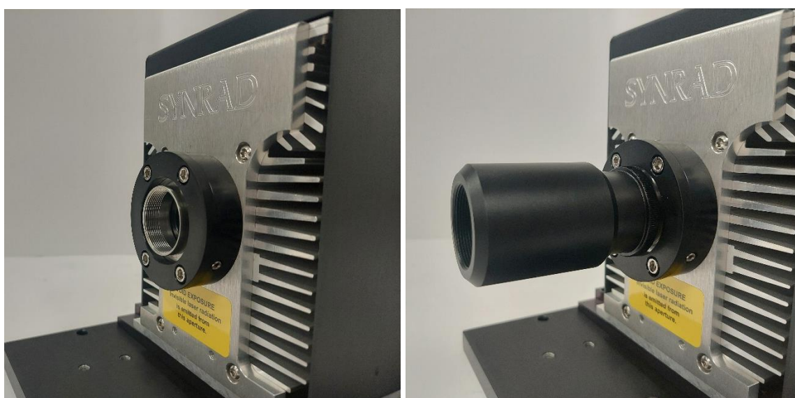
Figure 10: Translational beam expander mount – Beam expander mount fixed to the laser (Left); Beam expander mount with installed beam expander (Right).
